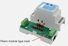
3. Insert the Fibaro<sup>®</sup> module firmly on the header pins up to the full depth and tighten <u>all</u> screws
