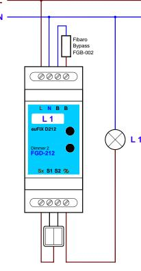
The descriptions of the screw terminals are printed on the adapter label. The sinusoid symbol with the arrow indicates the dimmer output, the letters "B" indicate contacts where the optional Fibaro Bypass FGB-002 can be connected.
