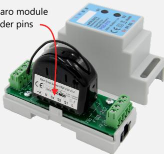
4. Close the cover, mount the Adapter on the DIN rail, connect the cables and label the module.
