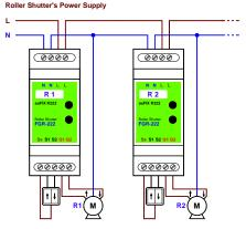
The descriptions of the screw terminals are printed on the adapter label. The "Q1" and "Q2" letters indicate the relays outputs.
