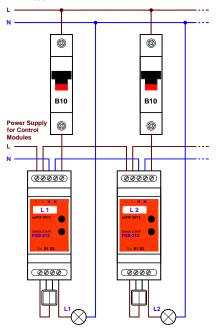
The descriptions of the screw terminals are printed on the adapter label. The letters "IN" indicate input for powering the load device. The "Q1" letters indicate the relay output.
