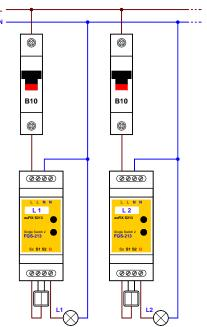
The descriptions of the screw terminals are printed on the adapter label. The "Q1" letters indicate the relay output.
