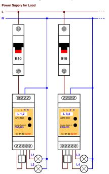
The descriptions of the screw terminals are printed on the adapter label. The "Q1" and "Q2" letters indicate the relays outputs.
