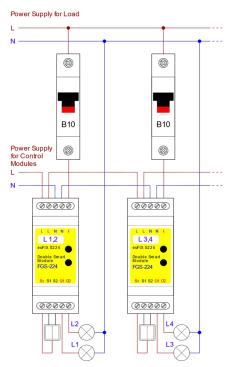
The descriptions of the screw terminals are printed on the adapter label. The letter "I" indicates input for powering the load devices. The "Q1" and "Q2" letters indicate the relays outputs.
