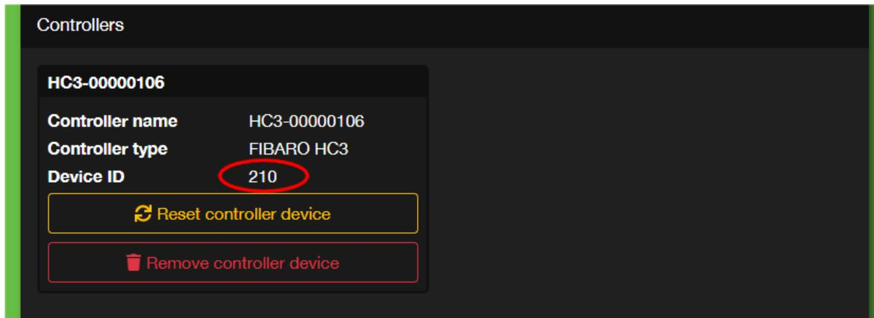
You can use that Device\_ID (in our example it is equal to **210**) in your scenes, maintaining the DALI luminaires in the Home Center environment. You will also find the global variable named "eu\_210\_level\_\*\*\*\*" containing the DALI luminaire dim level, that can be used for some useful numerical calculations.
