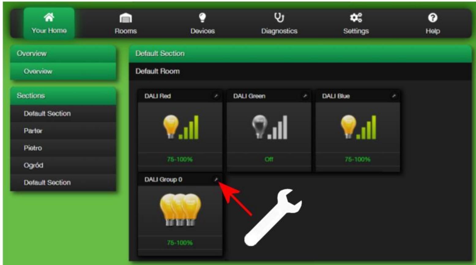
Clicking on the wrench symbol will open the detailed DALI device configuration, where you can test the luminaires or their group with the On/Off buttons and dim it with a slider:
