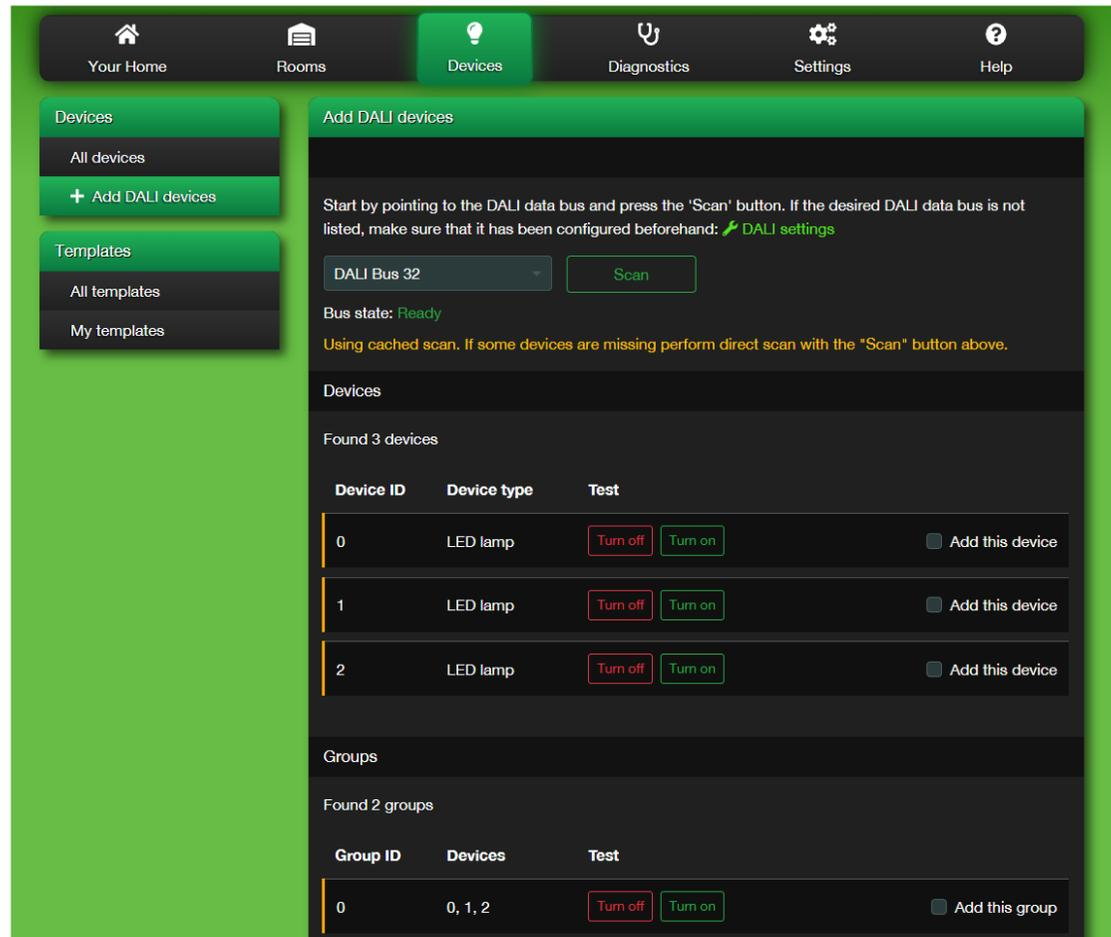
The only scenario where a new scan is required, is a recent change in the DALI bus configuration, e.g. adding new luminaires in the last few minutes. Please remember that **only one device can scan the DALI bus at one time**, so either euLINK or the DALI USB Programmer. Otherwise euLINK will report that the DALI bus is busy or inaccessible. Only a bus that is in the "Ready" state can be scanned. If the DALI bus is busy or disconnected, its status will be different.
