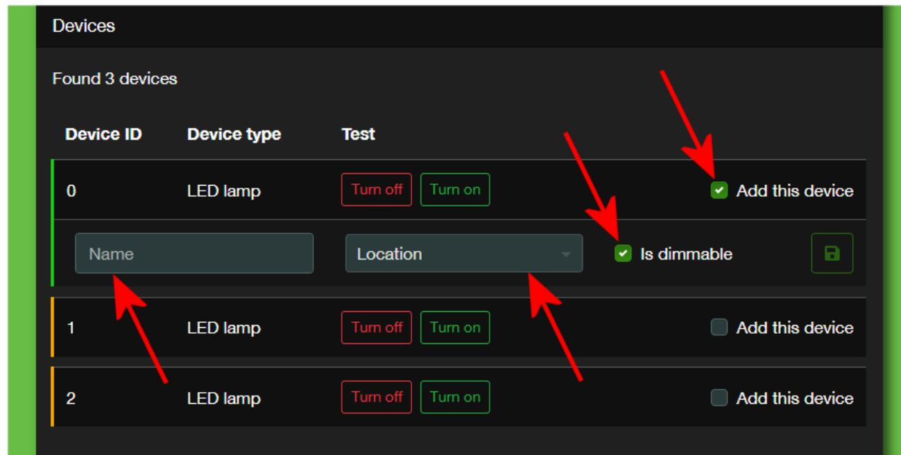
When the particular luminaire is named and assigned, it can be saved by pressing the diskette icon.
